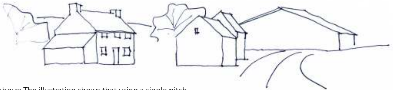
Above: The illustration shows that using a single pitch agricultural building is more dominant in the landscape
